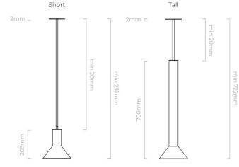
Drop: Minimum 23.cm (supplied with an adjustable 100cm drop rod)
